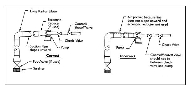
Figure 3.1 Inlet Piping
